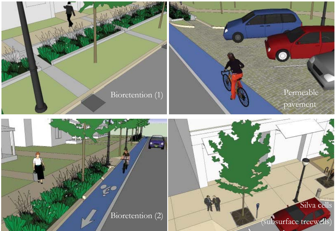
FIGURE 3. EXAMPLE STORMWATER TREATMENT METHODS
