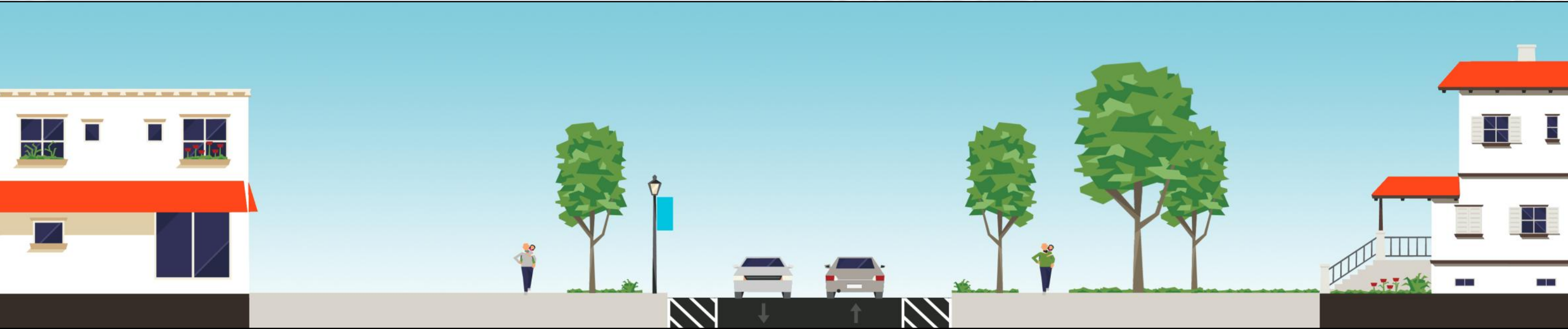
Cross-Section of Reconfigured Route 7 at Main Street with Planted Buffers and Traditional Lighting (view looking south)
