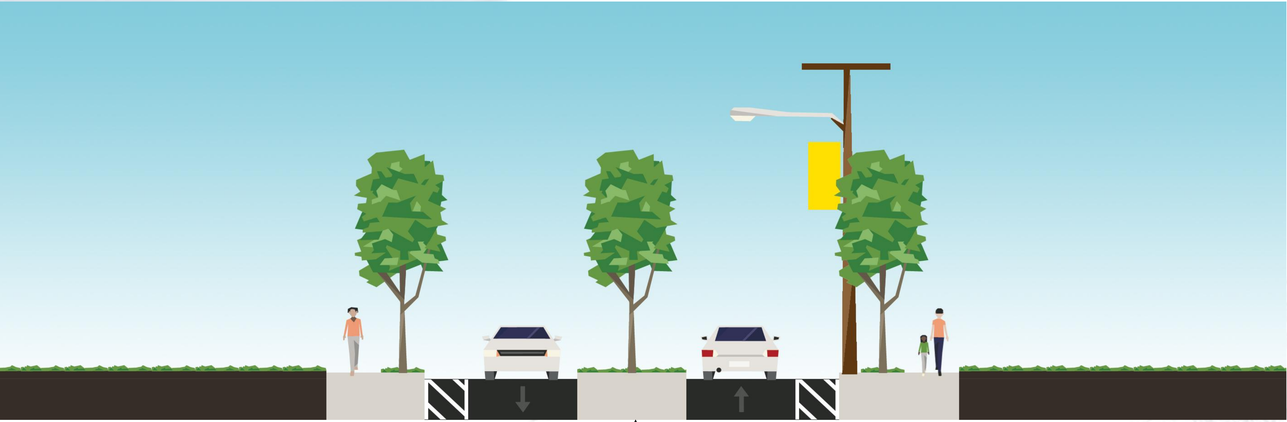
Planted median refuge island alternates with turn lanes to enable access to/from side streets
