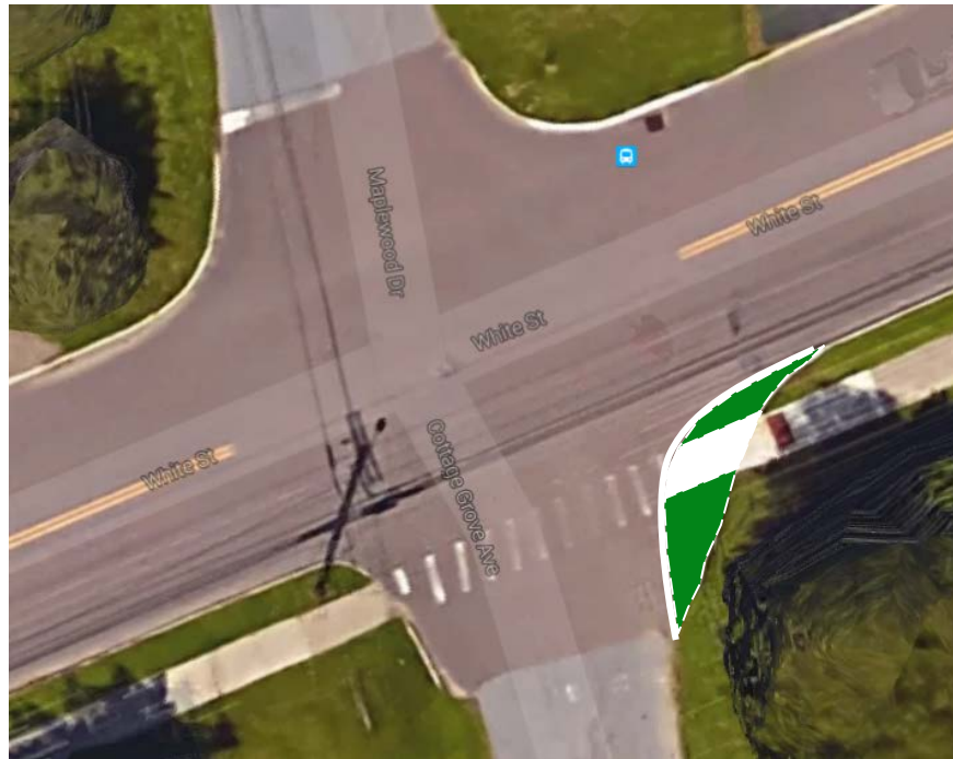
FIGURE 3-23: ILLUSTRATION OF CURB RADIUS REDUCTION AT INTERSECTION OF WHITE ST AND COTTAGE GROVE AVE
