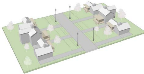
FIGURE 3-32: EXISTING FRONT YARDS WITH PORCHES AND 14' TALL STREET LIGHTS INSTALLED AT 40' ON CENTER
