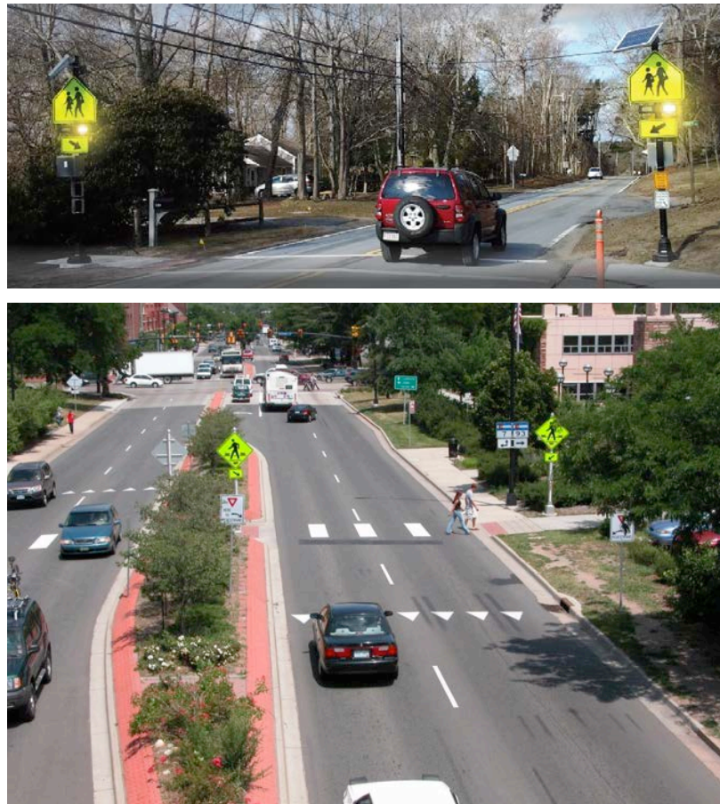
FIGURE 3-9: RECTANGULAR RAPID FLASHING BEACON AND ADVANCED YIELD LINE EXAMPLES
