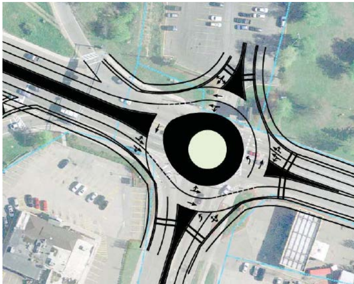
Figure 16. Proposed Roundabout Layout at Williston Road and Dorset Street
