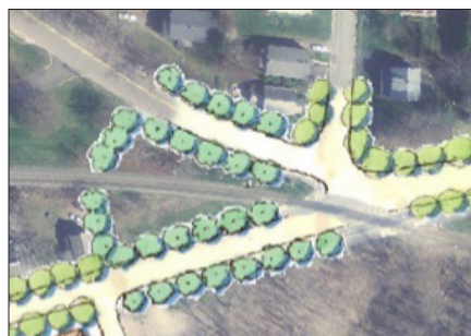
One option for re-routing and calming the Hood’s Crossing intersection, replacing the high-speed cross-merging movements with a new “T” intersection (signalized)
