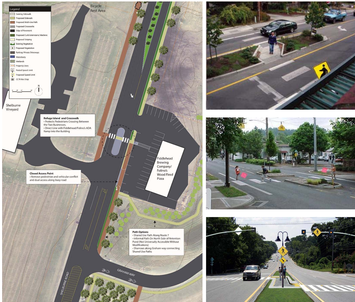
Figure 4.1: Proposed Crossing Design at Shelburne Vineyard on US Route 7 (left); examples of refuge islands (right)
