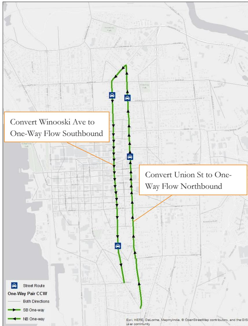
Conversion to one-way flow has the potential to free up pavement for alternate uses. While a one-way pair of bicycle lanes adjacent to vehicle lanes is one alternative for adding bicycle infrastructure in this scenario (Figure 12), it is not the only option, and alternate
