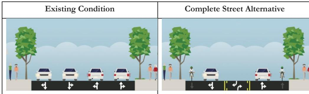
Keeping the current direction of travel and adding a bike lane from Main Street south to Maple Street requires removing parking on one side of Winooski Avenue and shifting travel lanes to the middle of the pavement to provide room for the bike lanes, but no vehicle travel lanes need to be removed (Figure 6).
