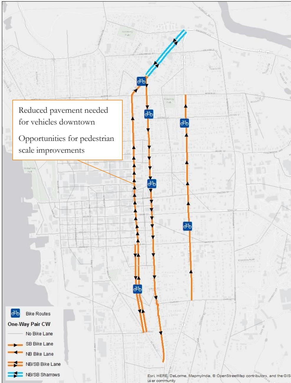
Figure 14 shows bicycle lanes adjacent to vehicle lanes and following the clockwise one-way pair flow direction. While this configuration is one alternative for adding bicycle infrastructure in this scenario, it is not the only option, and alternate configurations may be considered. Additionally, conversion to a one-way pair flow pattern may allow for additional parking or additional pedestrian scale improvement in some areas, especially downtown.
