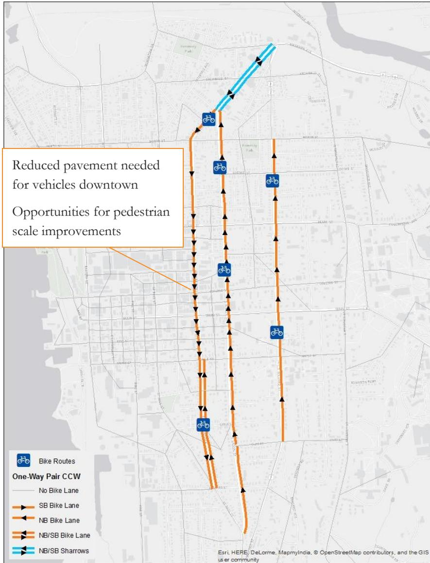
To assess traffic implications associated with this scenario in the Microsimulation model, the entire extent of Winooski Avenue is changed to one-way flow in the southbound direction and the entirety of Union Street is changed to one-way flow in the northbound direction. Two travel lanes are maintained on Winooski Avenue from Pearl Street to Main Street, as are turn lanes at key intersections. Signal timings are changed where necessary to accommodate the new traffic pattern.
