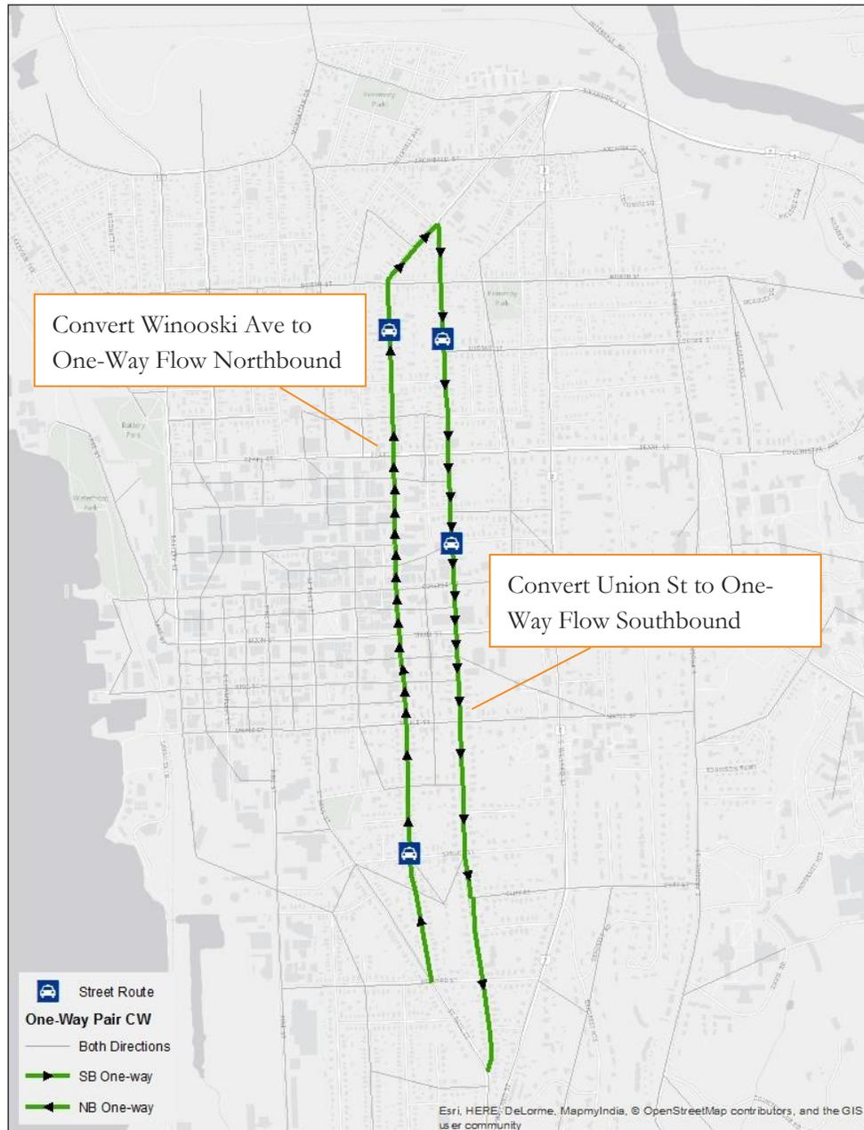
Flipping the direction of the existing one-way flow segments would require reconstruction of existing signalized intersections but would allow for right-turn movements to complete the one-way loop rather than left-turn movements. Right turn movements have been found to be more efficient, so this traffic pattern will enable more efficient traffic flow compared to a counter-clockwise flow.
