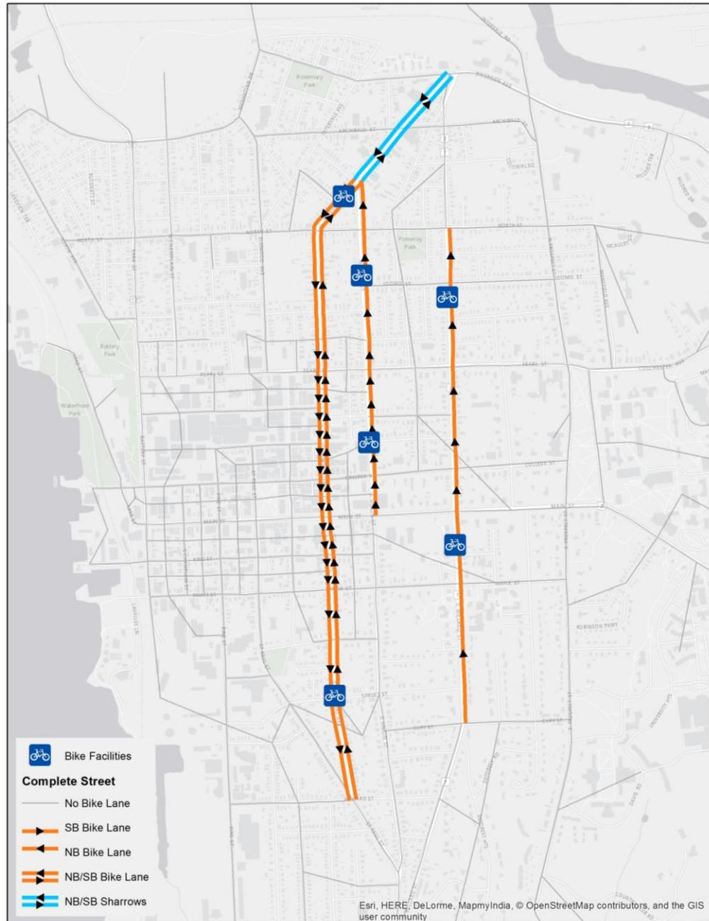
From Pearl Street south to Main Street, the entire curb-to-curb width of Winooski Avenue is currently dedicated to vehicular traffic. Bike lanes can be added by converting the four-lane cross section to three lanes (Figure 5).
