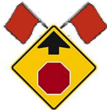
FIGURE 2: MUTCD R3-1 WITH TEMPORARY FLAGGING.
