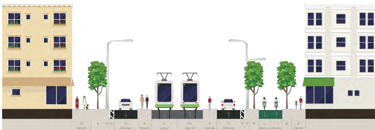
Figure 15: Williston Road Long-Term Corridor Cross-Section Option Four
