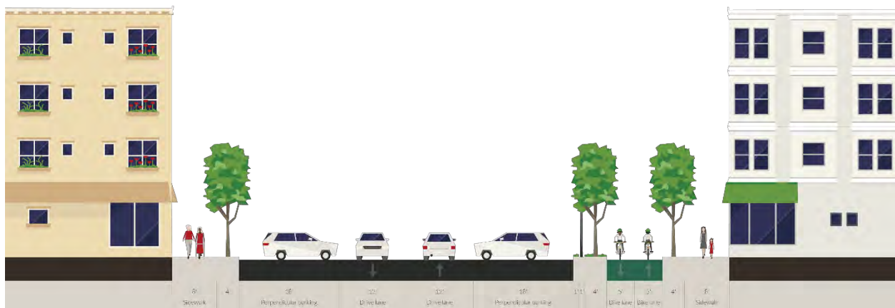
Figure 14: Williston Road Long-Term Corridor Cross-Section Option Three
