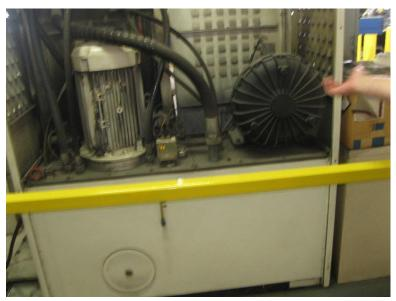
Photograph 2: Typical hydraulic reservoir and pump associated with production equipment.
