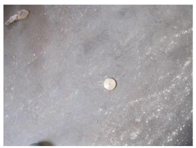
Photograph 4: Vapor pin installed in drum storage area.
