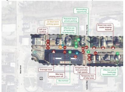
The group discussed the slip lane on Barlow Street and traffic exiting the parking garage. The slip lane also impedes safe navigation by cyclists. It was encouraged to investigate the need for the slip lane from a sight distance perspective.
