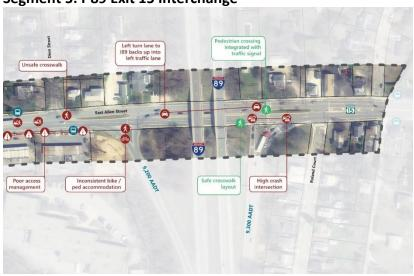
This segment is difficult for bicyclists due to confusing vehicle patterns. Sidewalks are narrow, in poor condition, and close to high-speed traffic. Traffic signal visibility is an issue for eastbound vehicles coming out of the underpass. Emergency responders noted there have been very serious crashes at this location in the past.
