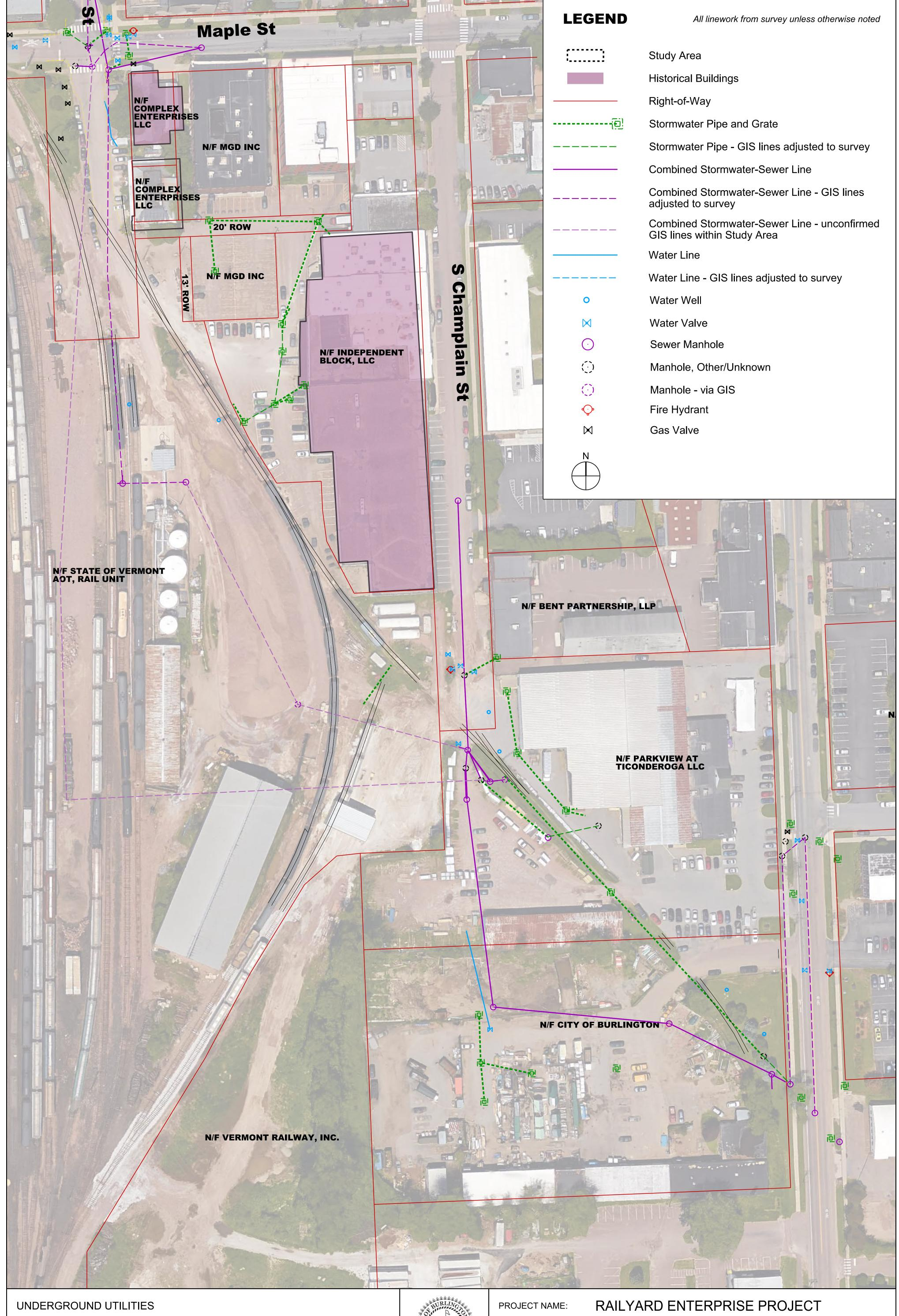
DESCRIPTION: Water, stormwater, sewer, and combined stormwater-sewer.
