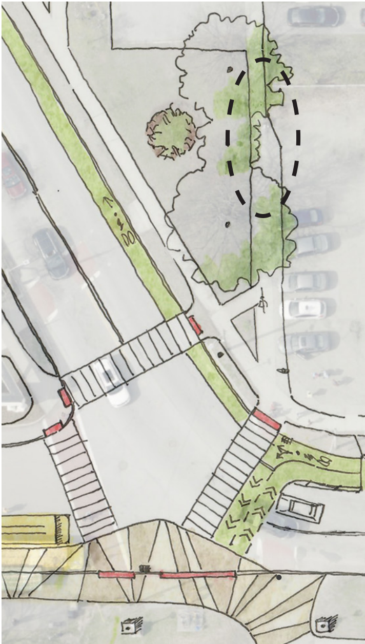
2 Widened sidewalk next to parking only, with width restriction at residential fence
