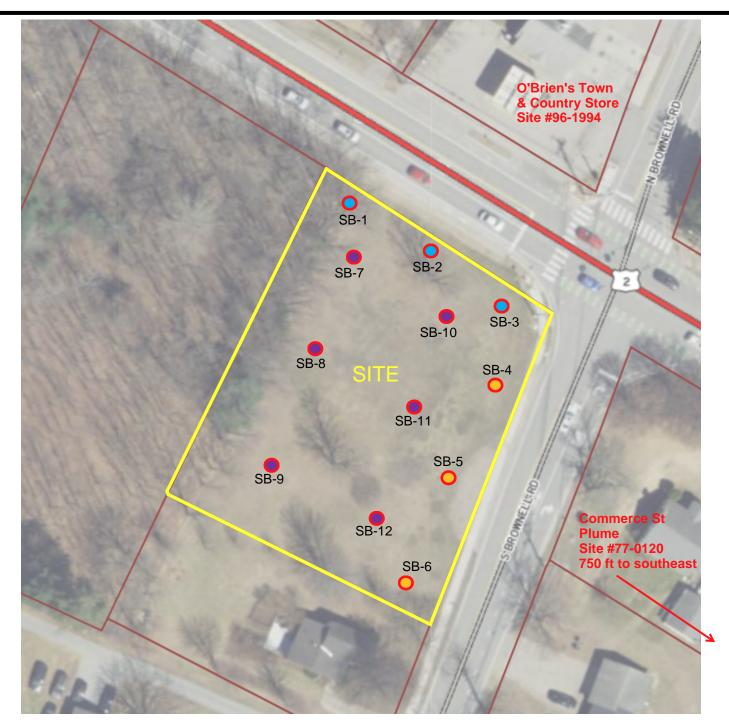
AOC #1 Proposed Soil Boring/Monitoring Well Location
